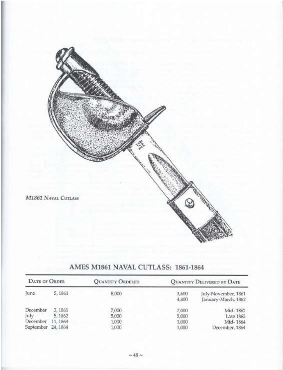
Figure 13 Ron Hickox Drawing of the M1861 Cutlass and Scabbard. Note the frog stub is mounted on a locket at the top of the scabbard.
